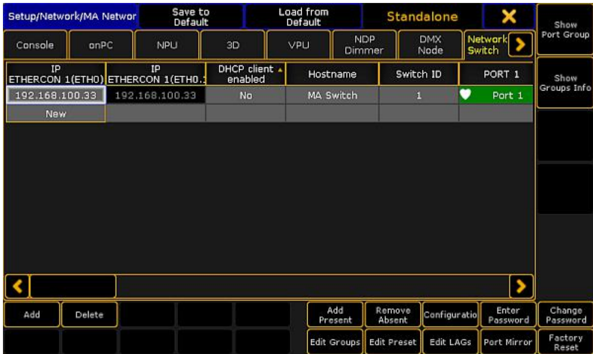
MA Network Configuration - Network Switch
