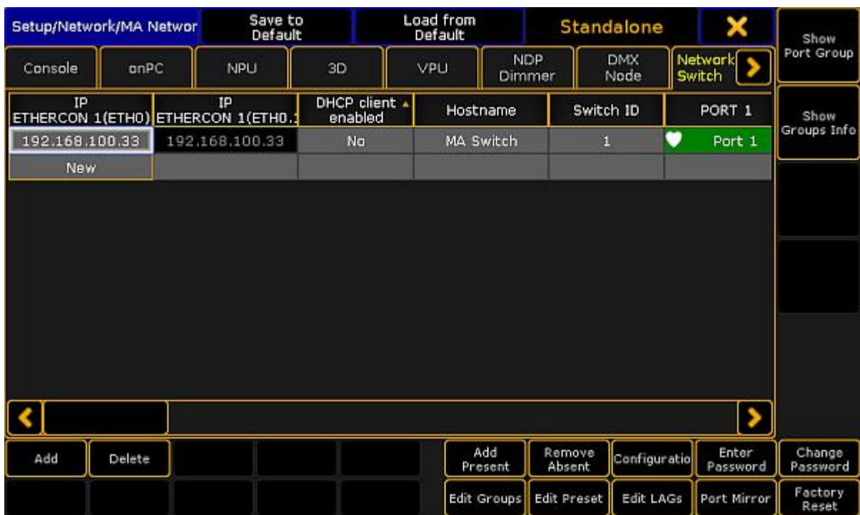
MA Network Configuration - Network Switch
