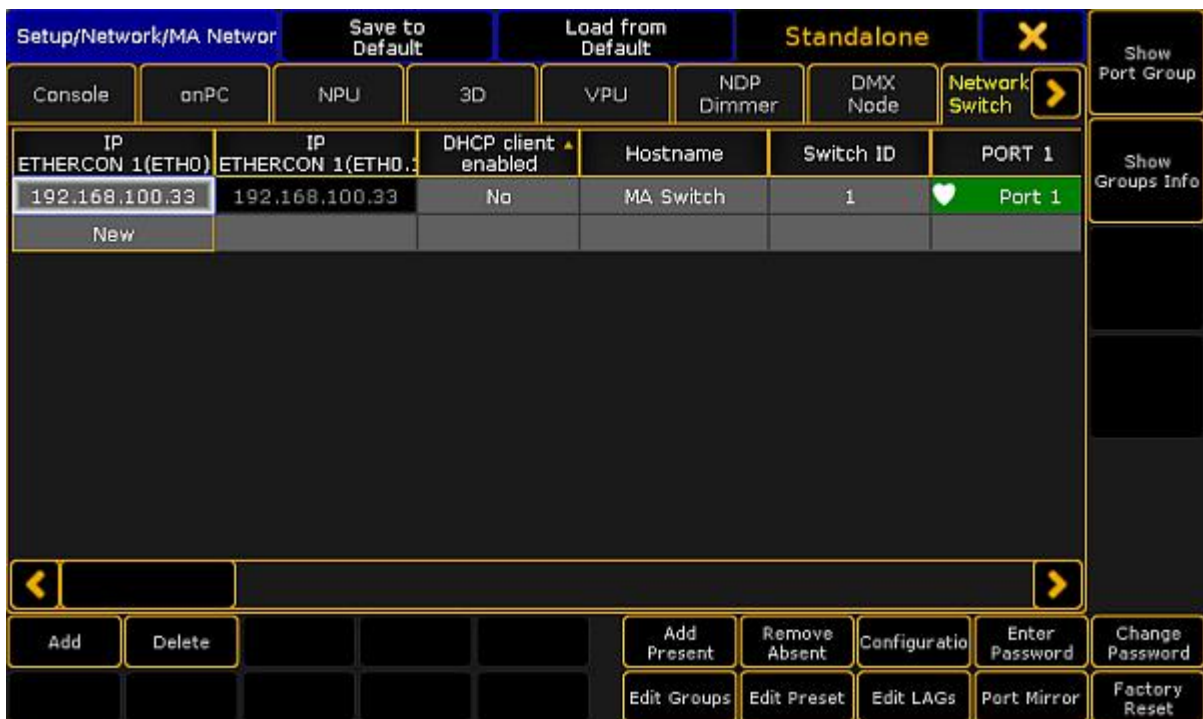
MA Network Configuration - Network Switch
