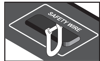
Figure 4: Safety wire attachment point
