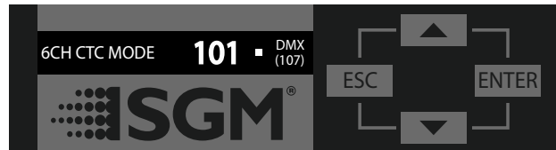
Figure 8: Q-7 OLED display and control panel
